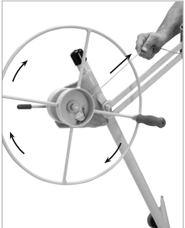
7. Feed the cable through the winch drum and secure it firmly behind the mooring tab as shown. Rotate the winch wheel in the direction indicated to take up the slack in the cable.
