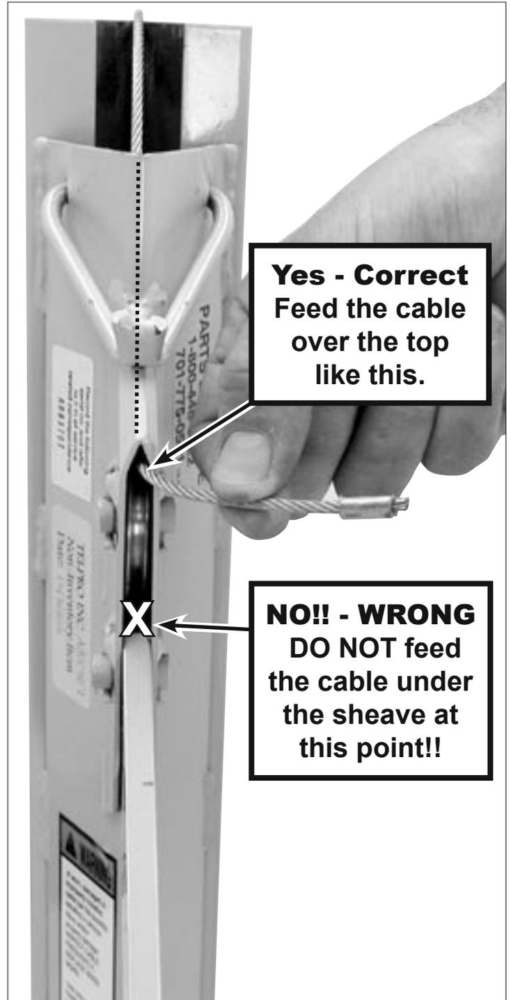
5. MAKE SURE that the cable feeds over the TOP of the cable sheave as shown in the above photo.
