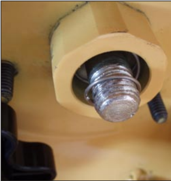
7) Install the winch handle spring as shown with the wide end in first and the narrow end out.
