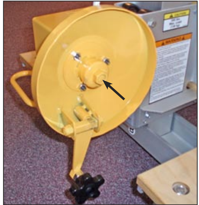
9) Install the Drill Drive™ winch hub ( NEVER try to use a drill to operate your Drill Drive™ winch system without this hub securely installed).
