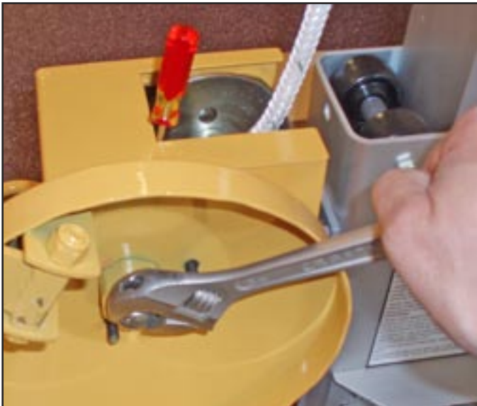
8) Install the winch nut and fasten securely in place. (You will find it helpful to lock the winch from rotating while tightening the winch nut by carefully inserting a small screw driver into the gear mechanism.)
