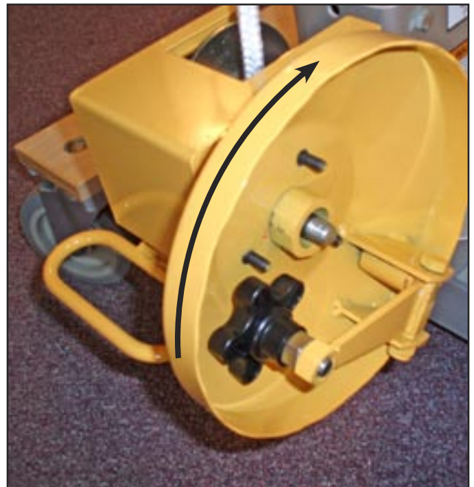
6) Install the Drill Drive™ winch handle by screwing it onto the winch drive shaft.
