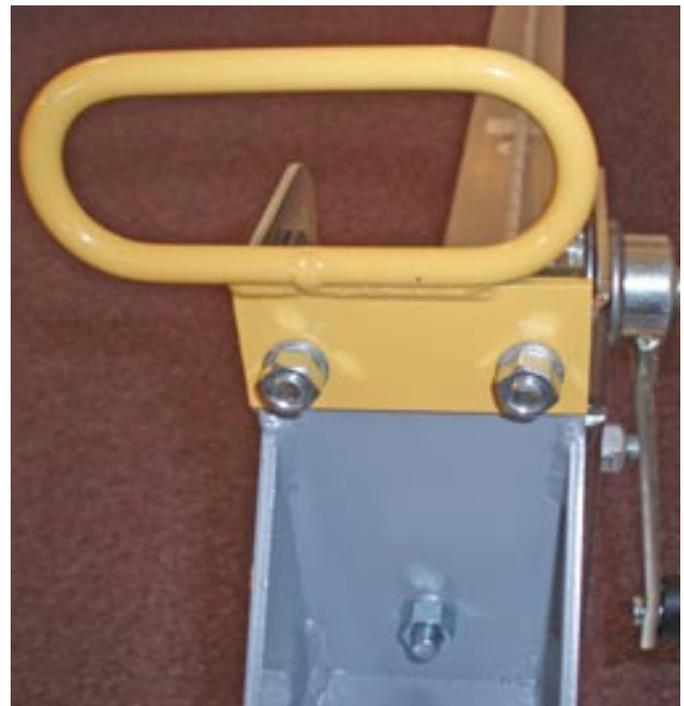
2) Install the grip handle as shown. Make sure the off set is to the left as shown to allow proper operation of the winch handle.
