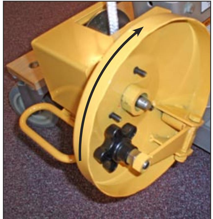
6) Install the Drill Drive™ winch handle by screwing it onto the winch drive shaft.
