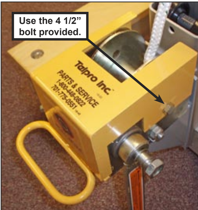
4) Install the winch guard and fasten in place with the 4 1/2" Bolt and lock nut provided for the winch spool axle bolt. (The bolt removed in step 3 above will be too short.) Tighten the lock nut enough to hold securely but not so much as to compress the winch spool housing.
