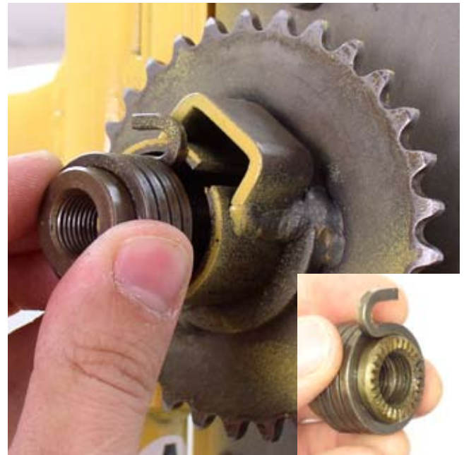
9) Thread the serrated bushing with the torsion spring onto the winch tube bolt until the torsion spring contacts the edge of the bushing housing as shown. IMPORTANT: Make sure the serrated end of the bushing goes on first and into the bushing housing as shown. Failure to install this bushing as shown will prevent correct assembly and operation of the reduction drive.
