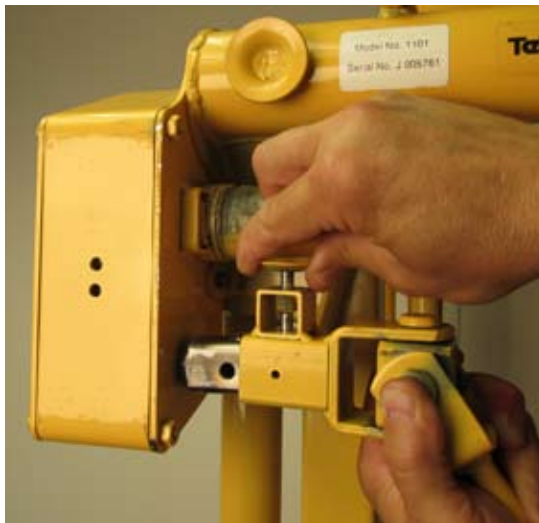
23) Attach crank handle to input shaft tube as shown. Secure in place with pull pin.
