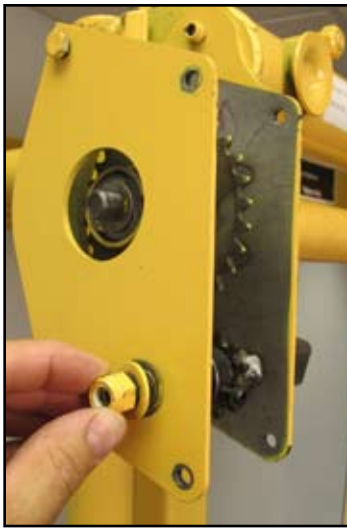
16) Install flat washer and 3/8" locknut on input shaft and tighten until it is snug.
