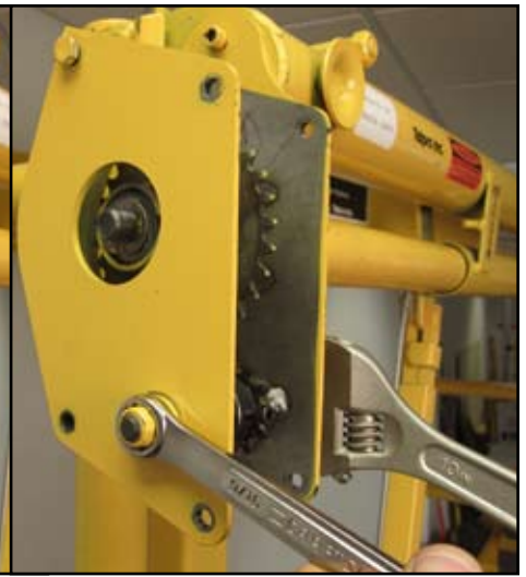
16) Install flat washer and 3/8" locknut on input shaft and tighten until it is snug.
