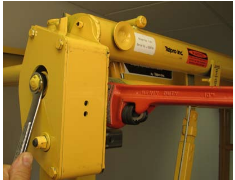
22) Tighten cap nut until snug. Control the rotation of the winch tube with a pipe wrench or pliers by gripping the welded areas as shown above and as in step 1.
