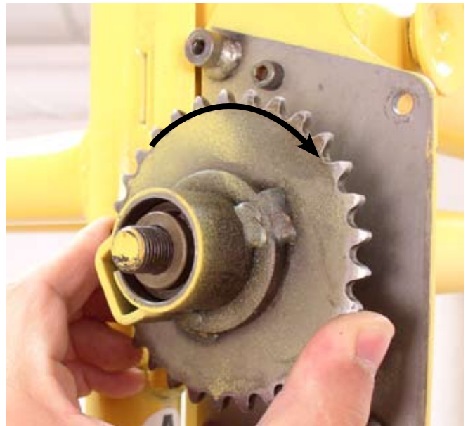
11) Rotate the sprocket clockwise until the serrated bushing is fully threaded onto the winch tube bolt.
