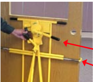
The Tilt Handle will adjust the door forward (4°) and backwards (12°) on either side of plumb.
