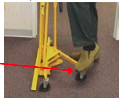
The Side Tilt Adjustment Wheel adjusts the door from Right (2°) to left (2°) on either side of plumb.
